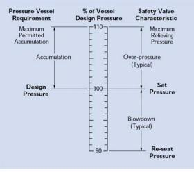
Note: System operating pressure must always be less than the re-seat pressure.
