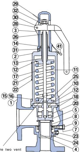
There are two vent holes to ensure spring chamber is at atmospheric pressure.
